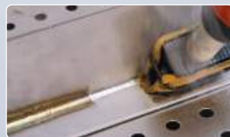
Old method: Welding seam cleaning with tampon
